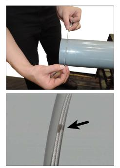
**11.** Once the groove is clean, check the groove diameter ("C" dimension). A pipe diameter cable, supplied with the tool, is the recommended method for checking the "C" dimension. Refer to the wide angle view and close-up shown above.
