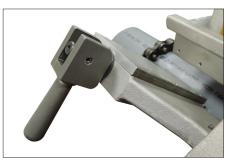
**3.** Put the toggle clamps in the disengaged position.
