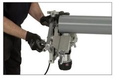
5. Tighten the arm locking knobs to handtight. Do not over-tighten.
