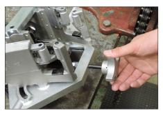
7. Using the motor carriage adjustment knob, verify that the bit is positioned high enough to clear the pipe OD when mounting the tool. Rotate the knob counterclockwise to raise the bit and clockwise to lower the bit.
