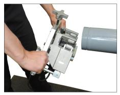
**9.** Verify that the tool bit is clear of the pipe and cannot damage the pipe "A" dimension (groove location) during removal.
