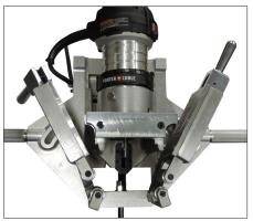
**4.** The 2–4 inch arms must be mounted on the tool in a specific orientation. Match the "A" or "B" etched on the arm with the corresponding letter on the tool body, then insert the arms into the tool body so that the matching letters face each other.
