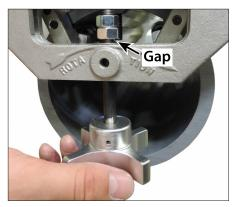
4. Turn the motor carriage adjustment knob clockwise to lower the bit into the pipe until the depth stop rests on the pipe. When the depth stop rests on the pipe, the adjustment knob will turn easily and a gap will develop between the nut and the washer.
