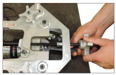
**11.** Tighten the depth stop locking nut to hand-tight. Do not overtighten.
