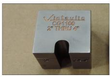
1. Retrieve the 2" THRU 4" alignment block. Alignment blocks are etched with the pipe size in inches.
