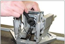
While pressing the spindle lock button, use the <sup>5</sup>/<sub>4</sub>-inch wrench to loosen the collet. Remove the 6–12 inch bit.
