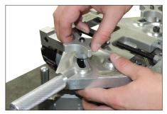
2. Unscrew and remove the arm locking knobs.
