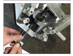
**9b.** To change the cutter bit location, use a flat-head screwdriver to twist the depth adjustment screw until the tip of the bit rests just below or meets the selected line on the alignment block.
