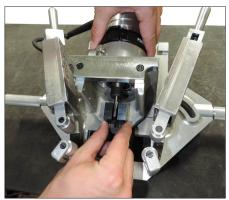
8. Align the notch on the back of the alignment block with the depth stop behind the bit. Slide the alignment block over the depth stop until fully seated.
