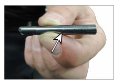
2b. Take note of the line etched on the base of the bit. This marks the minimum depth of insertion when installing the bit into the tool.
