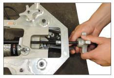
4. Use the 7/16-inch wrench to loosen the depth stop locking nut.
