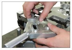
2. Unscrew and remove the arm locking knobs.
