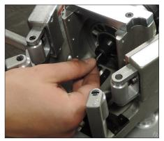
**5.** Insert the 2–4 inch cutter bit into the collet to just past the minimum insertion depth.
