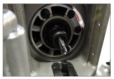
7. Verify that the cutter bit is inserted deeply enough for the etched line to be partially or fully covered by the collet.
