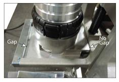
**3.** Adjust the 'A' adjustment screw so that the back edge of the motor fixture is drawn firmly against the motor carriage with no gap. There should be a gap between the front edge of the motor fixture and the motor fixture stop.
