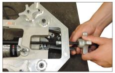
**11.** Tighten the depth stop locking nut until hand-tight. Do not overtighten.
