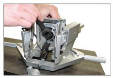
6. While pressing the spindle lock button, use the %-inch wrench to tighten the collet until hand-tight. Do not overtighten.
