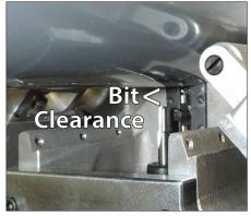
7. Turn the motor carriage adjustment knob counterclockwise to lift the bit until it will clear the pipe when removed.
