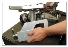
**4.** The 6–12 inch arms are interchangeable and may be mounted on the tool in either orientation. Insert the arms into the body of the tool.
