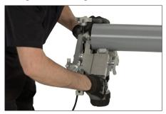
**6.** Put the toggle clamps in the engaged position, then hand tighten until the OD and ID rollers are against on the pipe. Do not overtighten.
