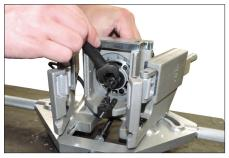
While pressing the spindle lock button, use the %-inch wrench to loosen the collet. Remove the 2–4 inch bit.
