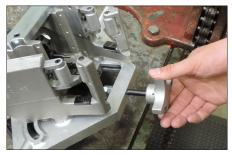
7. Using the motor carriage adjustment knob, verify that the bit is positioned high enough to clear the pipe OD when mounting the tool. Rotate the knob counterclockwise to raise the bit and clockwise to lower the bit.
