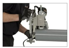
7. Push the tool through one complete clockwise rotation to check for obstructions and to allow the tool to track onto the pipe. Verify that the tool tracks onto the pipe, and that the tool moves freely throughout the entire rotation.
