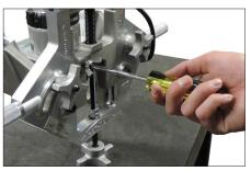
Using a flat-head screwdriver, rotate the "A" adjustment screw counterclockwise to adjust the groove location.
