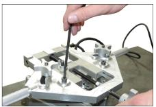
**1.** Loosen and remove the shoulder bolts using the provided hex key.
