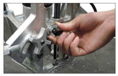
**1.** Loosen the wing nut on the "A" adjustment screw, located on the front of the tool.
