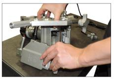
**3.** Pull the 2–4 inch arms straight out from the body of the tool. When not in use, store the arms in the provided tool bag.
