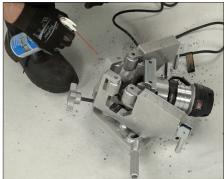
Clean chips from the tool with a soft brush or compressed air.
