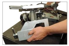
**3.** Pull the 6–12 inch arms straight out from the body of the tool. When not in use, store the arms in the provided tool bag.
