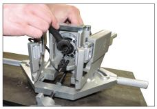
6. While pressing the spindle lock button, use the <sup>5</sup>/<sub>8</sub>-inch wrench to tighten the collet to hand-tight. Do not overtighten.
