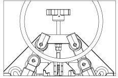
**4.** Lift the tool with both hands on the handles. The bit should face towards the pipe.
