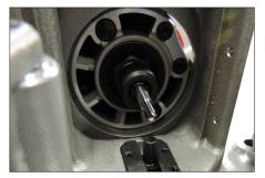
7. Verify that the cutter bit is inserted deeply enough for the etched line to be partially or fully covered by the collet.
