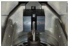
**9a.** Select the appropriate cutter bit location by matching the pipe size to the corresponding line on the alignment block.
