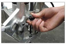
**4.** Tighten the wing nut on the "A" adjustment screw, located on the front of the tool.
