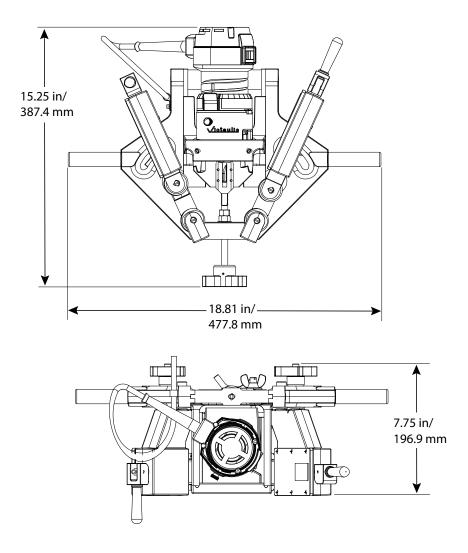
Tool weight is 17.2 pounds/7.8 kilograms when using 2-4" arms, and 21.3 pounds/9.6 kilograms when using 6-12" arms. Tool weight includes the tool assembly, motor, handles, and arms.
