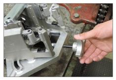
Using the motor carriage adjustment knob, verify that the bit is positioned high enough to clear the pipe OD when mounting the tool. Rotate the knob counterclockwise to raise the bit and clockwise to lower the bit.
