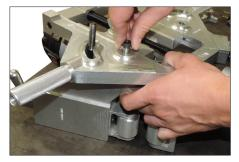
6. Replace and tighten the shoulder bolts to finger-tight.
