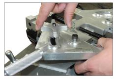
Replace the arm locking knobs and screw down until the arms are secure against the body of the tool.
