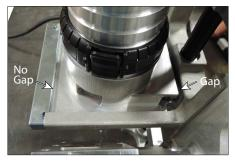
**3.** Adjust the "A" adjustment screw so that the front edge of the motor fixture is drawn firmly against the motor fixture stop with no gap. There should be a gap between the back edge of the motor fixture and the motor carriage.
