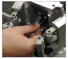
**5.** Insert the 6–12 inch cutter bit into the collet to just past the minimum insertion depth.
